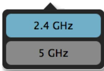
**Note:** when the Access Point is set to 5GHz equipment used to connect must also function at 5GHz. A 5GHz connection will generally result in less interference from other equipment, but will also not penetrate solid objects as effectively.
