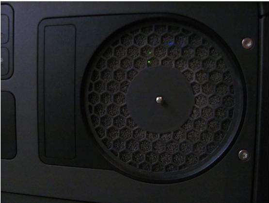
With the air intake grill removed the filter material is visible. Carefully remove the filter material:
