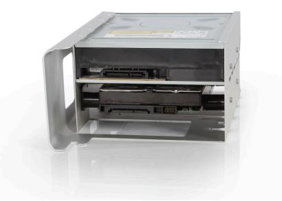
Then slide the optical drive carrier halfway back into the drive bay and reconnect the power and ribbon cables.
