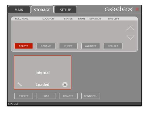
Now click the CREATE button and input a name for the Roll that will be created across the disks. This Roll is simply to identify the storage when it is loaded in Codex software. Shots that are cloned from a Datapack or Capture Drive will maintain their original Roll metadata when copied.
