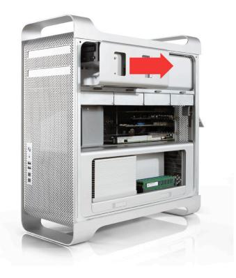
Disconnect the power and ribbon cables from the optical drive and remove the carrier fully.
