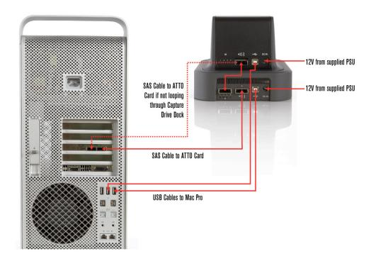
The diagram below shows the cabling setup with the ATTO H6F0 configuration.
