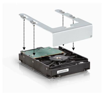
Refit the Hard disk drive carriers into the machine by sliding onto the guides until they snap into place.
