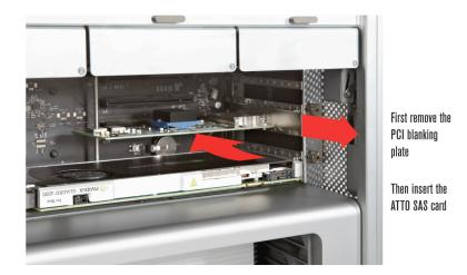
Secure the card by re-fitting the PCI bracket.
