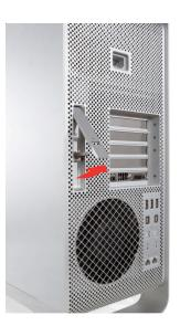
Lay the computer flat so that the open side faces upwards, and work in a well lit environment. After installing hardware refit the side panel and close the latch on the rear of the computer.
