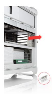
Remove the PCI blanking plate for the slot you intend to use for the ATTO SAS card. Do not move the system graphics card that is already installed.
