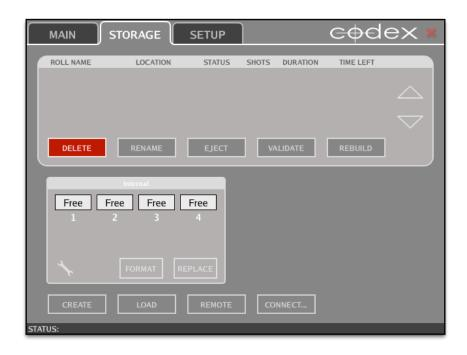
If the boxes that represent each drive are grey in colour and do not say Free then they have not been formatted correctly (which means there is still a GUID partition table on the disk), or there is no disk fitted in that position.
