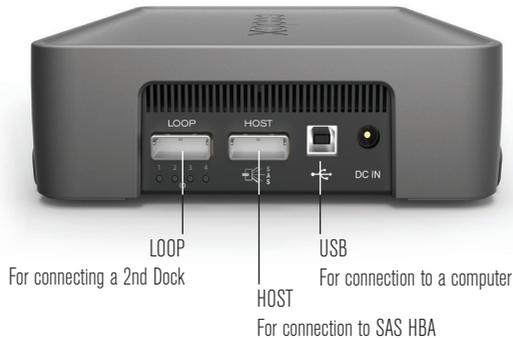
The ID LED on the rear of the Dock indicates the number assigned to it by the Codex software, as multiple Docks can be connected to one Mac.
