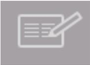
**Filecard** - to view and edit clip metadata. Click the first clip then click this button. Use the Up and Down arrows on your keyboard to move between clips. Make changes and then click the checkbox to save. The **Log Note** field contains details of any issues detected during recording.
