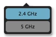
Note: when the Access Point is set to 5GHz, equipment that can only operate up to 2.4GHz will not be able to connect.
