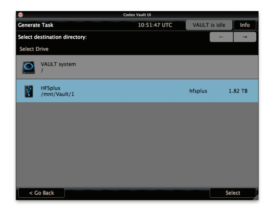
A top level directory will always be created on the drive used for the Generate Task, which is given a unique name based on the date and time the task was started in the following format:
