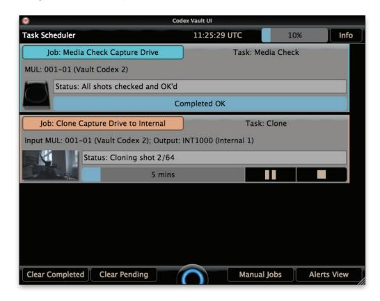
Jobs can be paused or stopped if required using the buttons next to the progress bar for an individual job.
