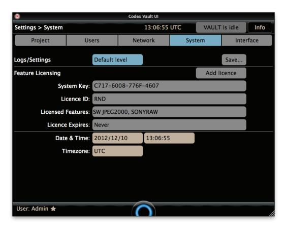
This screen is used for saving system log files, adding feature licences, and adjusting the system date/time.
