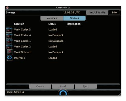
The Create option can be used on unformatted Codex media to apply a name and specify the RAID type in order that it can be used by the Vault, Onboard S recorder or Alexa XT.
