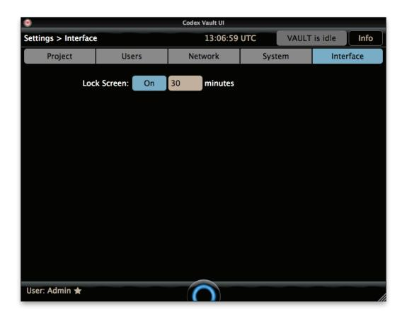
On this screen the Vault can be set to automatically lock after a specified amount of time. Once the Vault is locked then a user account and password is required to log back in.
