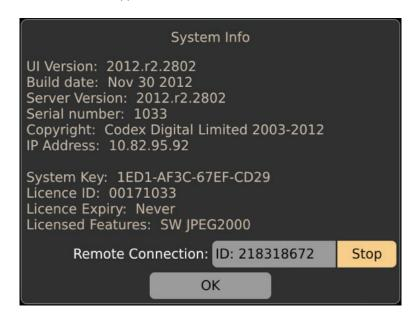
With the Vault connected to a network with internet access click Start and a 9 digit ID should be displayed in the Remote Connection box. From another computer you can then run the TeamViewer software and enter this ID and the password **codex** to connect to the Vault.
