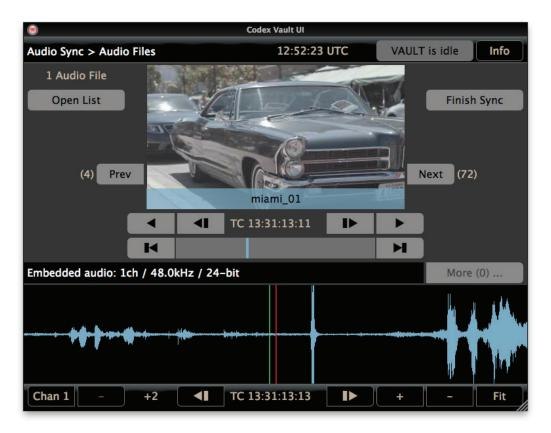
Press the **Play shot** button to check the sync has been successful. You can step through using the **Forward 1 frame** and **Back 1 frame** buttons to confirm this with accuracy and monitor via the headphone output of the Vault.
