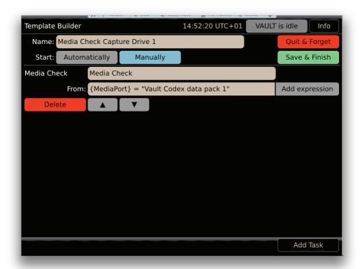
Most Tasks require a "From:' expression that specifies the {MediaPort} - physical location of the media - for the Task. So in this case the Media Check will run on the media that is loaded in the CODEX 1 port.
