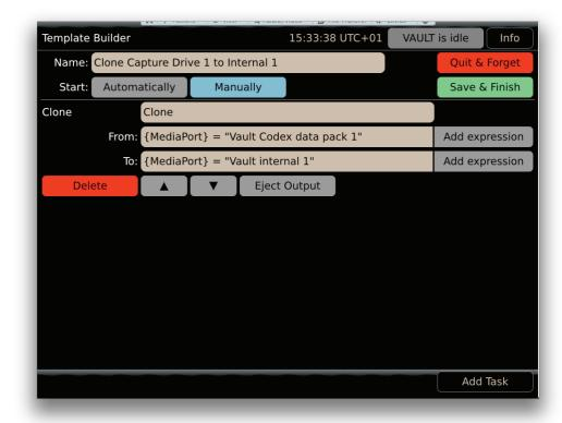
This Task will clone material from the media loaded in the CODEX 1 port to the Internal 1 (Storage Module).
