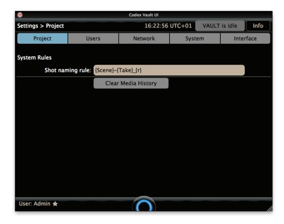
The Clear Media History button should only be used before a new project begins, as detailed in the earlier section 'Preparing the Vault for a new project'.
