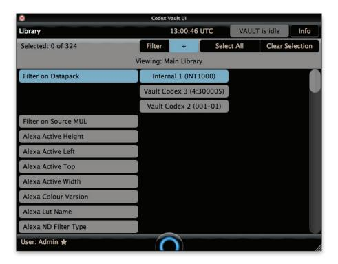
At the top of the list are the options to **Filter on Datapack** (physical media) and **Filter on Source MUL** (if there is material from multiple MULs on a single media – this is most likely with the Internal Storage):
