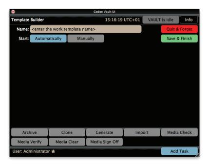
At the top of the screen you can edit the name of the Work Template, normally to something self explanatory, e.g. Check and Archive Capture Drive.
