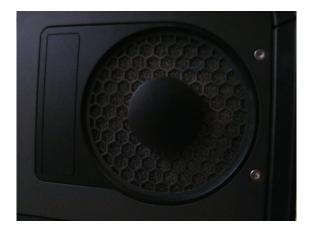
Remove the air intake grill. It is clipped in place but can be freed with a small amount of wiggling. A pair of needlenose pliers can be used for this, holding the grill near to the central disk:
