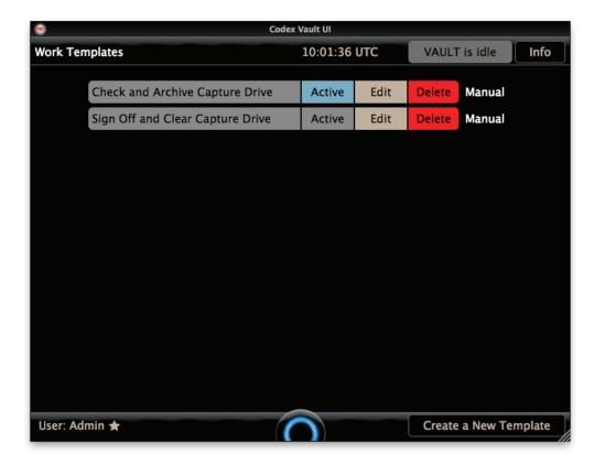
From this screen you can select if a Work Template is Active. If a Work Template is set to start Automatically then it will only be able to start when it is Active. If a Work Template is set to start Manually then it will only be shown on the Manual Jobs screen when it is Active.
