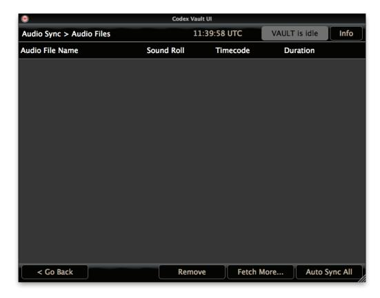
Click the Fetch More... button to load files from an attached device, e.g. USB drive.
