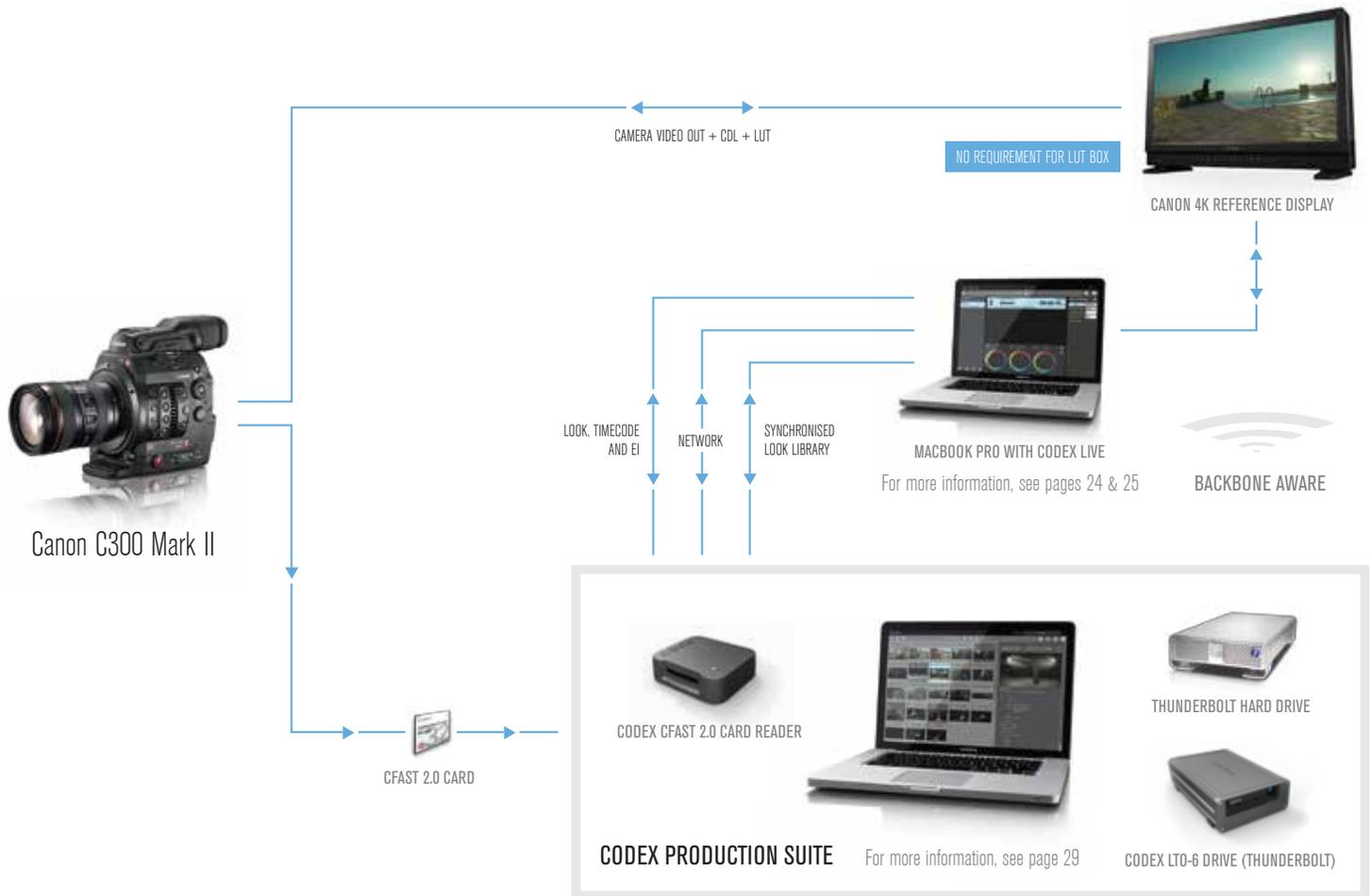
Codex fully supports Canon's new XF-AVC format, a MPEG-4 AVC/H.264 video compression format which provides a high data compression rate without sacrificing image quality. Combine this with an efficient, reliable workflow, and you have an ideal scenario for productions of every size and budget. Codex Production Suite on a MacBook Pro is a fully-featured dailies and archiving system in a small footprint that can travel wherever you need to be.
