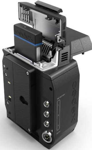
The door of the V-RAW Recorder is located on the top. Pull the lever on the door towards the rear of the V-RAW Recorder to release the door and lift it to the fully open position.
