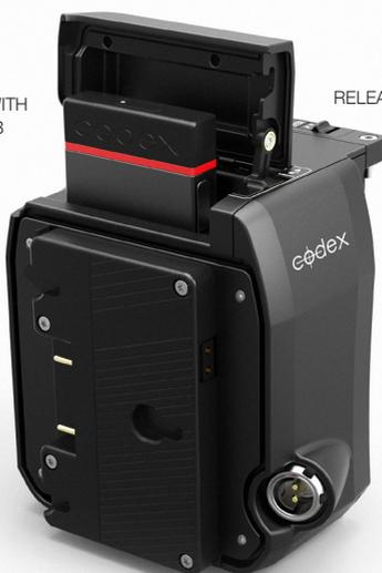
The media access door of the CDX-36150 is located on the top. Slide the release catch next to the door to open.
