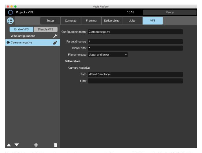
The VFS (Virtual File System) screen is where you set up the file types available from the 'Codex VFS'. On Mac OS X the 'Codex VFS' is a drive that appears on the Desktop. On Vault S/XL-Series the 'codexvfs' is a network shared folder, accessible via Samba and NFS.
