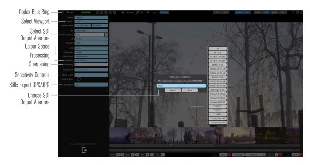
The output resolution can be set from the **SDI** menu. Once an SDI output device is successfully detected, then options for **Aperture**, **Link** and **Bit Depth** will appear.
