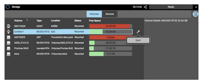
The Volumes tab shows each loaded storage media (camera media, hard drive, LTFS tape) with details of the filesystem type, location, and space remaining. Select media and click the wrench to Eject.
