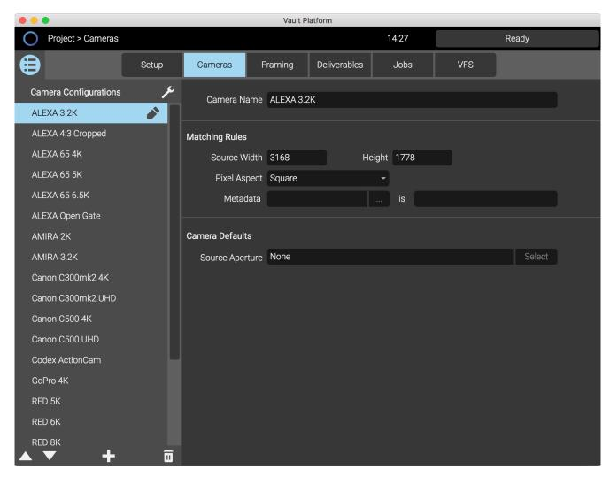
There are a range of preset Camera Configurations available, but you can also add your own as required. The preset Cameras Configurations need to be edited by adding the relevant Source Aperture (region of interest) for your production.
