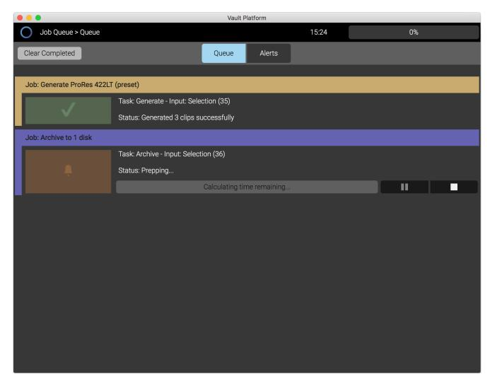
The Job Queue screen shows the progress of jobs that are running. Jobs can be paused and stopped with the buttons as required. If user input is required, for example to choose the target directory, then an Alert will be shown. The Job Queue displays when a task has completed, or information if any errors occur during a task.
