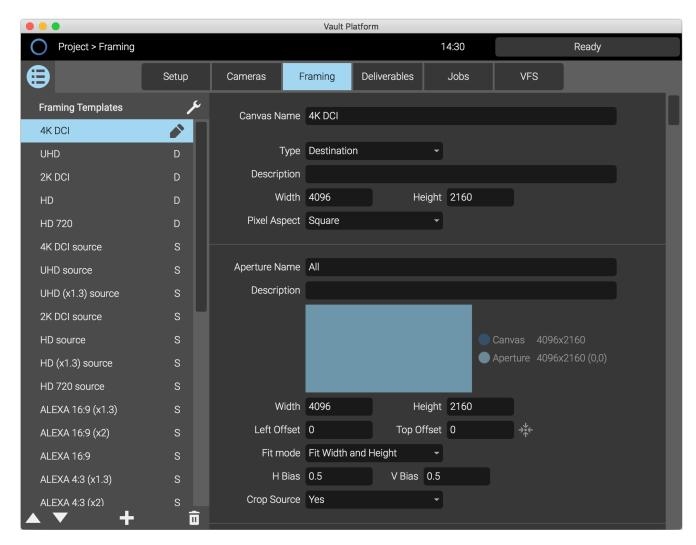
The Framing screen contains presets to cover the most common requirements. The left panel shows the full list of Framing Templates.
