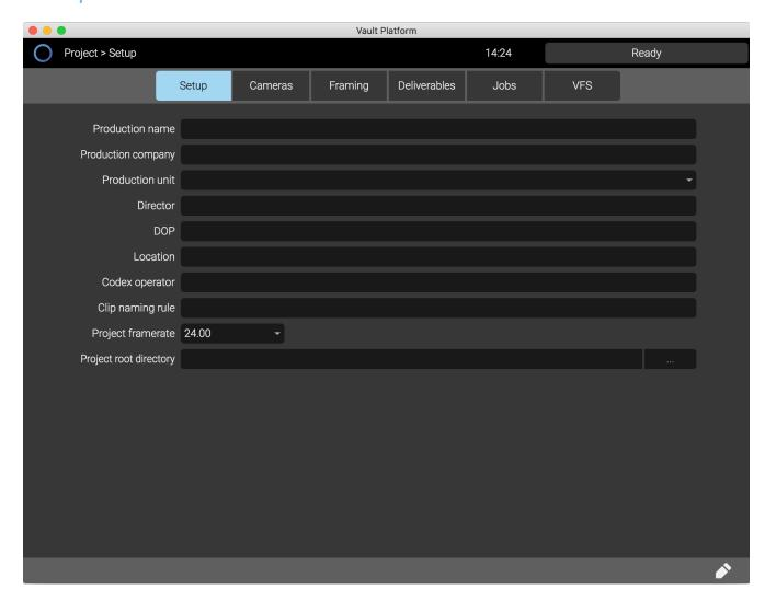
The Setup screen is where you can input production details. This can be applied as metadata to clips during a Media Check task with the 'Apply Project Defaults' button.
