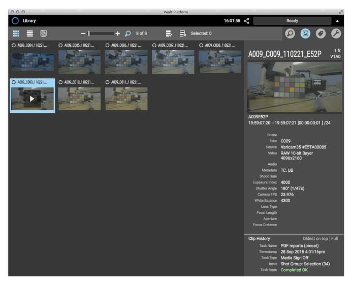
Important metadata such as Scene, Take, Format, EI, WB, and Shutter Angle is shown, as well as clip duration in frames (e.g. 1423 fr) and as timecode at the Project frame rate (e.g. [00:00:59:07] / 24).
