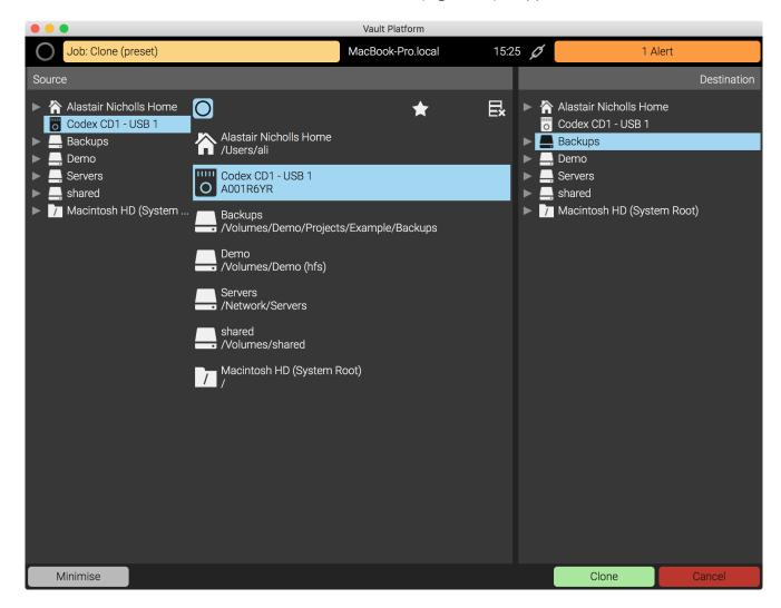
The left hand panel contains a tree view that can be used to navigate through the filesystem. The central panel is where the source is selected, and right hand panel is where the destination is selected.
