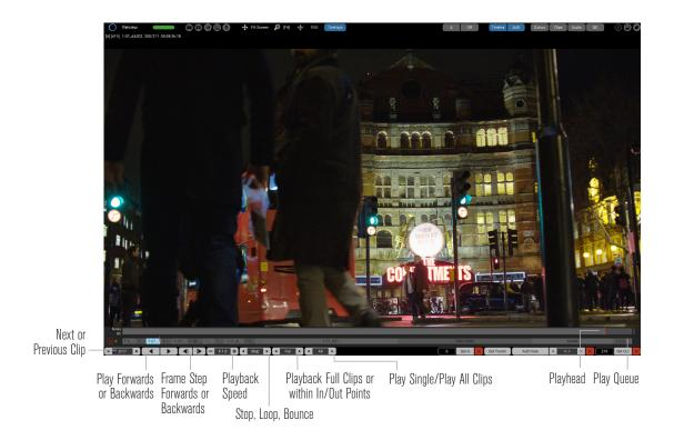
The transport controls are located at the bottom of the screen.
